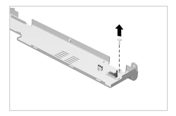
Figure 5-26. Removing the Display Switch Button
